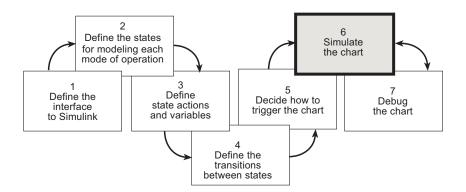
In phase 6 of this workflow, you *simulate the chart* to test its behavior. During simulation, you can *animate* Stateflow charts to highlight states and transitions as they execute.
