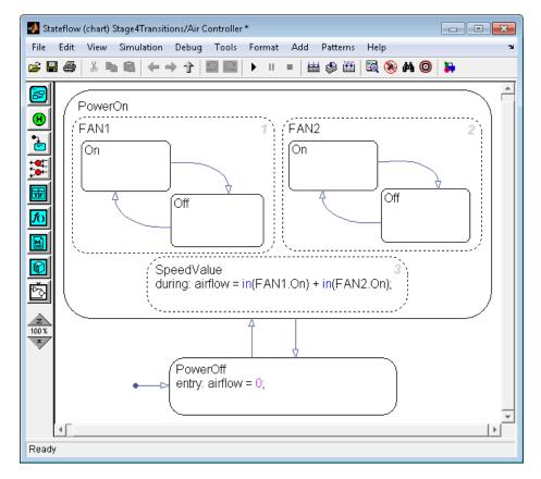
**5** Repeat the same procedure to add default transitions at the top edges of FAN1.Off and FAN2.Off.
