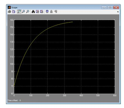
Note in the output display pane of the debugger that temp has risen to over 157 degrees. The Scope displays the temperature pattern:
