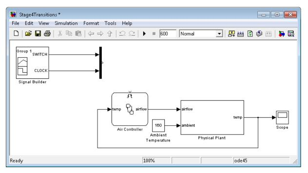
When you define one or more input events for a chart, Stateflow software adds a single trigger port to the block. External Simulink blocks can trigger the input events via a signal or vector of signals connected to the trigger port.
