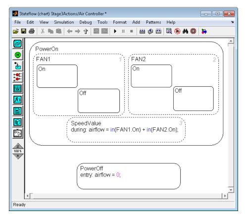
The Boolean expression in(FAN1.0n) is true — and its value equals 1 — if the On state of FAN1 is active. If FAN1 is not on — that is, its Off state is active or power is off — then in(FAN1.0n) equals 0. Similarly, the value of in (FAN2.0n) represents whether FAN2 is on or off. Therefore, the sum of these Boolean expressions indicates whether 0, 1, or 2 fans are operating during each time step.
