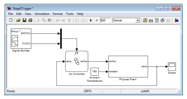
The output signal of the Mux block connects to the input trigger port of the Stateflow block. Your model should look like this:
