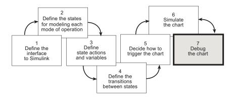
In phase 7 of this workflow, you *debug the chart*. In Chapter 8, "Simulating the Chart", you learned how to use the debugger for setting breakpoints and observing data. In this chapter, you will learn how Stateflow software detects errors and provides diagnostic assistance.
