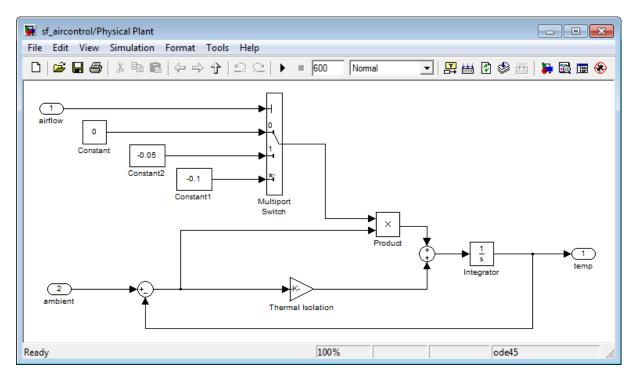
In this model, the internal temperature of the plant attempts to rise to achieve steady state with the ambient air temperature, set at a constant 160 degrees (as shown in "How the Stateflow Chart Works with the Simulink Model" on page 2-6). The rate at which the internal temperature rises depends in part on the degree of thermal isolation in the plant and the amount of cooling activity.
