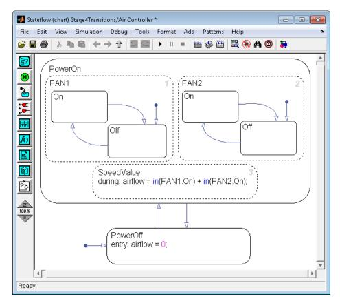
**Tip** The location of the tail of a default transition determines the state it activates. Therefore, make sure that your default transition fits completely inside the parent of the state that it activates. In the Air Controller chart pictured above, notice that the default transition for FAN1.Off correctly resides inside the parent state, FAN1. Now consider this chart:
